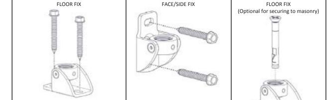
NOTE: Ensure fasteners suit substrate application Max fastener size #10, Max Dynabolt Size: M6
