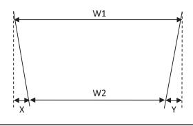
If W2 < W1, by a value of: 0-20mm, Proceed to Part B (W1 = Blind Width) 20+, Consider corrective action to square installation space
